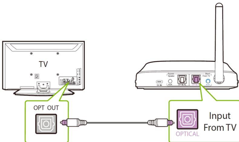
*NOTE: Most TVs support audio output through only one digital output port at a time, so if your TV's HDMI ARC port is in use, the optical port may be disabled. You can either unplug the HDMI ARC device, or try connecting the transmitter via RCA / AUX.*
