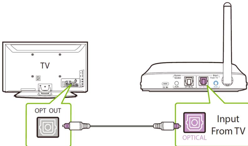
*NOTE: Most TVs support audio output through only one digital output port at a time, so if your TV's HDMI ARC port is in use, the optical port may be disabled. You can either unplug the HDMI ARC device, or try connecting the transmitter via RCA / AUX.*
